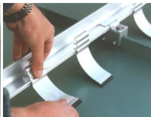
"toe" must engage panel surface
